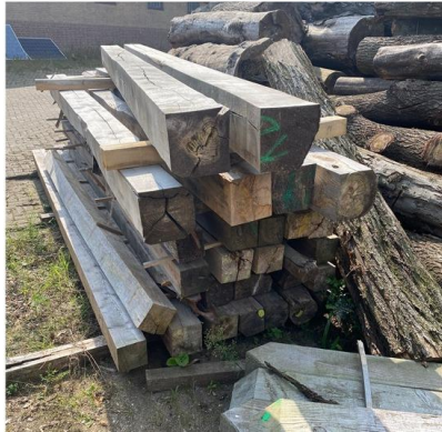
Figure 4: Reused elm timber beams and urban wood at the circular sawmill
