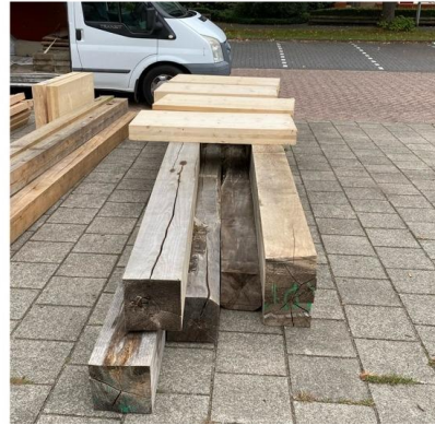
Figure 5: Reused elm timber beams and CLT blocks on site
