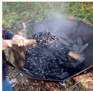
Figure 9: Producing biochar from construction off-cuts
